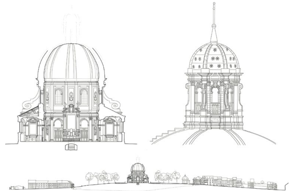
Fig. 6. Collage of the different scale levels: Urban cross-section (bottom), Cross section of the central building (left), north façade of the Lantern (right). ©Lehrstuhl für Architekturgeschichte, RWTH Aachen University (Anke Naujokat, Survey Team) Lehrstuhl für Architekturgeschichte, RWTH Aachen University (Anina Janich, Tim Scheuer)
